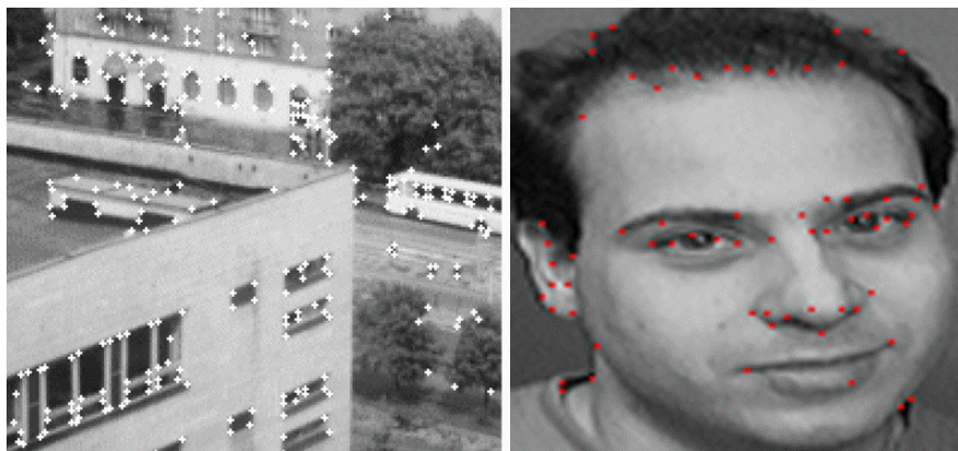
Figure 10. Detected corners in an image obtained from a CCD camera.
