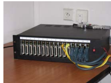
Fig. 4. Our Implementation of Hardware-based Crossconnect for Serial WAN Ports
